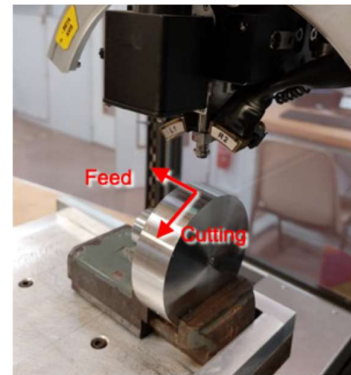
Fig.4. Specimen mounted in X-ray diffraction machine (Proto®).
